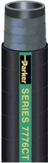
Series 7776CT is excellent for high-pressure top deck reel and platform type fueling equipment. The proprietary rubber compounds enable this hose to stay flexible in extreme low temperatures. The premium nitrile tube minimizes permeation and will not contaminate product going through the hose. Also suitable for defueling service at low pressures (suction/vacuum rating to 8 in. Hg).
