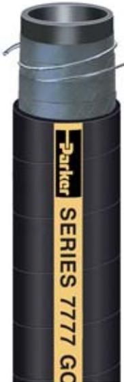
Series 7777 acts as a flexible connection for jet fuel supplied through an adjustable elevated service platform, called a jac-riser, connected to a mobile dispenser cart that is supplied by an in-ground hydrant system. The dual wire helix provides flexibility, kink resistance and full suction capability for both fueling and defueling/unloading service. The premium nitrile tube minimizes permeation and will not contaminate product going through the hose.
