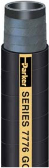
Series 7776 is excellent for high-pressure top deck reel and platform type fueling equipment. The premium nitrile tube minimizes permeation and will not contaminate product going through the hose. Also suitable for defueling service at low pressures (suction/vacuum rating to 8 in. Hg).
